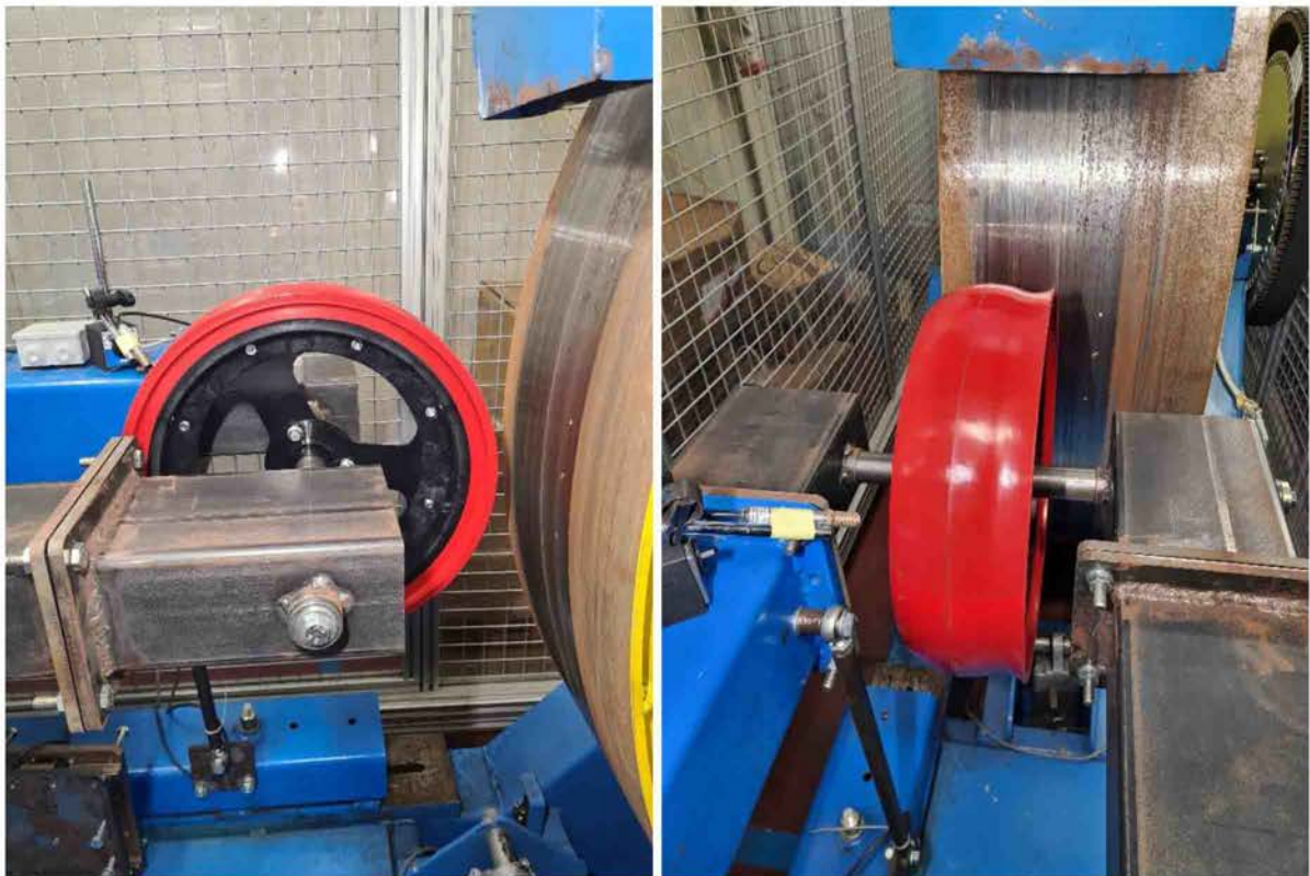
Figure 2 Sample mounted on the radial load test bench
